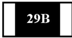
$1.96\text{K}\Omega = 196 \times 10^1 \Omega = 29\text{B}$
